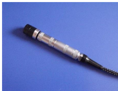
Figure 1. Developed high-frequency INDETEC EC probe
